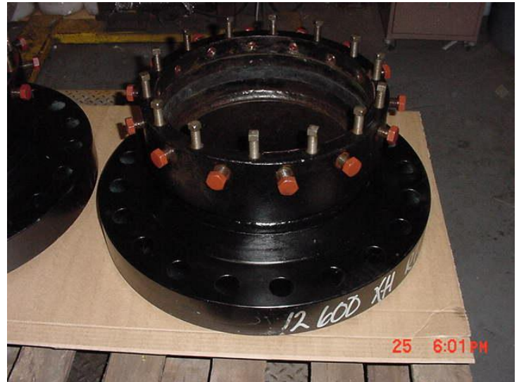
12" ANSI Class 600 - Flanged End Connector. Dual Seals, Sub-sea Crude Oil Service located at Gulf of Mexico.
