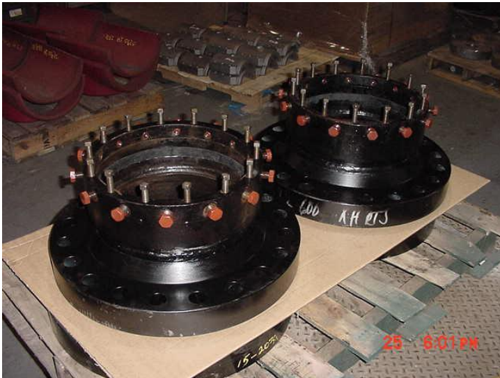
12" ANSI Class 600 - Flanged End Connector. Dual Seals, Sub-sea Crude Oil Service located at Gulf of Mexico.
